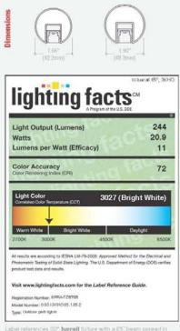
High Output 3000K. Lighting Facts for additional beam and light output levels may be obtained from io Lighting
